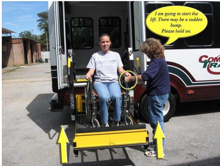
Check the roll stop to ensure it is locked in 'up' position. After making certain roll stop is locked, continue raising the lift platform to van floor level. Secure pendant in its holder.
