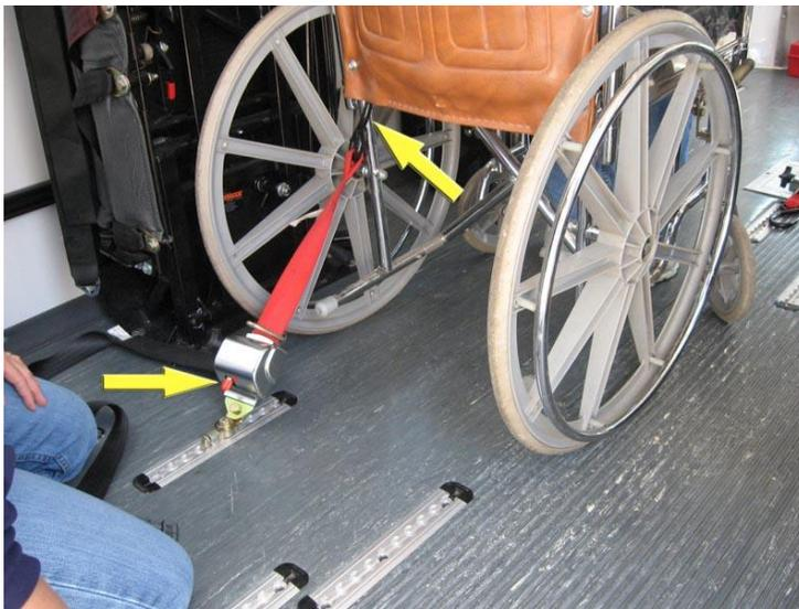
Attach the tie-down straps to each of the corners of the wheelchair by attaching the hook at one end of the strap to the wheelchair.
