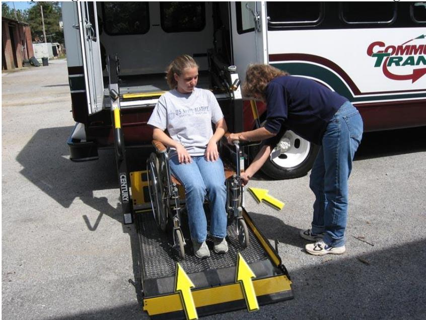
Roll the passenger backwards onto the lift facing away from the van and secure both brakes on the wheelchair. The platform roll stop is not designed to stop a fast moving wheelchair. *Note: If the passenger wishes to board the lift facing the vehicle they must be allowed to do so.*
