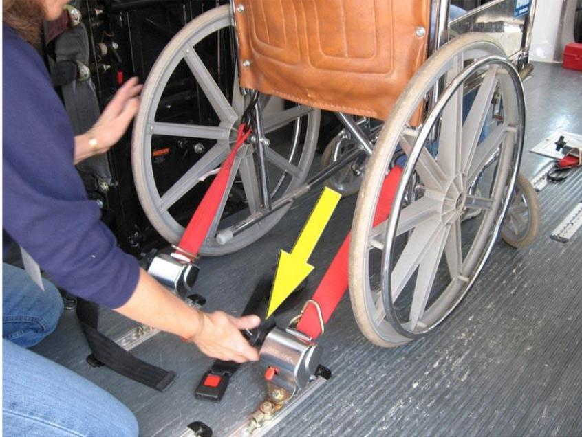
Attach the shoulder belt on the wall mount and place the shoulder belt diagonally across the middle of the passenger's shoulder and sternum area of the chest.
